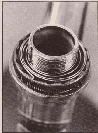
See how one end of that spring catches an indentation on the inside of the top bearing race, while the other end hooks into the notch in the fork crown? That's how the Epoch headset's self-adjusting feature works — and it DOES work. We never had to touch the adjustment.
