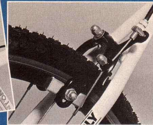
Dia-Compe 890 caliper, Araya 7X aluminum rims, and Cheng Shin knobs. The brakes work good, the rims stayed round (even after MUCH abuse), and the tires grip passably well.
