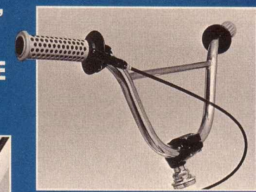
When we tested the DB Super Viper back in the February '85 issue, we let Cosmo have the bars 'cause they fit him purr-fect. Well, he's got another set of bars to add to his collection 'cause we replaced 'em with a set of Galindos that are much wider than the 22 3/8 inch width of these dudes. His new pair will definitely last longer than the previous set, though. These 'uns are totally chrome-moly.
