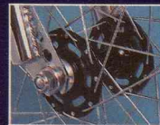
Precision sealed-bearing SunTour hubs
