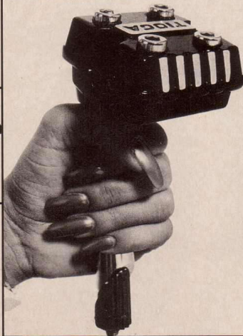
Forged aluminum clamps and a chrome-moly shaft make up the Tioga Task Force stem.
