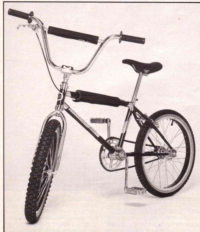
Scorpion's brazed racer—the triple-lugged chrome-moly Super Team.
