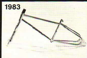
1983 Lil' Hole Shot Mini-frame—2 lbs. 14 oz. Mini Forks—1 lb. 5 oz. New lighter weight for '83! New BB, new seat post w/built in seat clamps.
