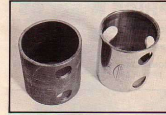
This is TRICK. On the left, your ordinary bottom bracket. On the right, the new Red Line double-butted and drilled-out jobber. Red Line gave the head tube the same treatment and saved almost a half pound per bike with no apparent loss in strength or rigidity.
