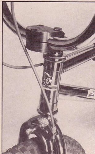
The Pro-Am head tube has machined flanges for added strength at the bearings. Quality stuff.
