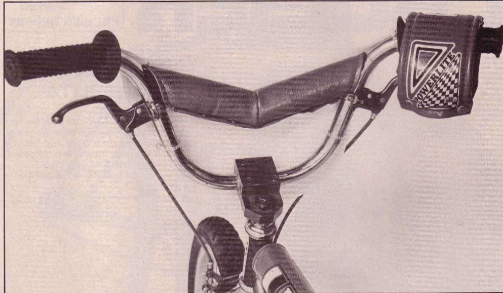
Micro Lines and a Tuf-Neck or Pro-Neck are the inside hot tip for cruiser racing.
