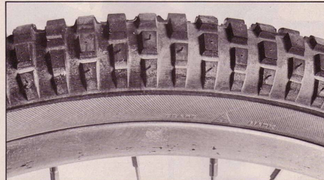
Compare the scoopers on the sides of the knobs on the Comp III (on the top) to the knob pattern on the Comp II: There's more gription when you accelerate, and more grab when you lay it over.
