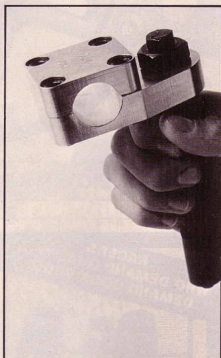
This is the Pro-Neck Beach Cruiser stem. It has a one inch hole to accept flared bars.
