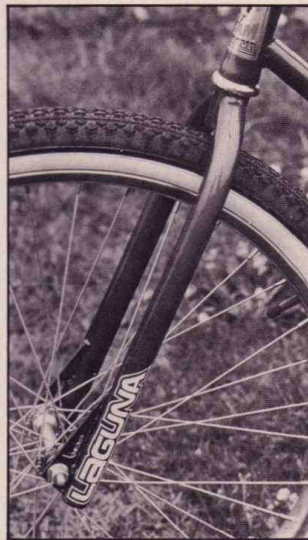
In the steering department the Laguna is graced with leading axle forks made of chrome-moly.
