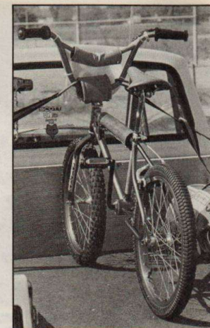
The Clinton machine: Diamond Back frame and forks, Red Line Micro Line bars, Shimano SR gooseneck, Araya square shoulder rims. Shimano alloy front hub and quick change rear hub, blue plastic seat, MKS pedals, Takagi 7 inch forged cranks, Haro number plate, Grab-On grips, Tournay side pull callipers with Mathauser shoes, 2.125 Cheng Shin in front, 1.75 Cycle Pro skinwall in back (with the sidewall painted black), 44 tooth front sprocket and a 16 tooth rear.
