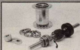
Remove the stuff in the other photo, add a Shimano 3-speed clutch spring (arrow), and you've got a freewheeling hub.
