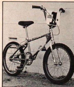
The Encinas machine; Mongoose frame, Dura-Ace cranks, 2.125 Cheng Shin front tire, 1.75 Cheng Shin rear, Red Line "V" bars, Araya alloy rims, Shimano hubs, Shimano freewheel, Tange forks, Oakley II grips, Shimano lever and calipers.
