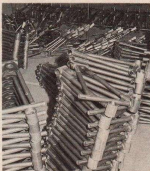
Front and rear triangles, welded and waiting to meet their master (jig).
