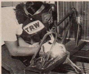
Front and rear triangles getting the business in the master jig. Next stop: the painters or platers.
