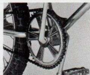
The old standard: 6 1/2-inch Schwinn diamonds. These cranks are reasonably light and almost indestructible. They are heat-treated, of course.
