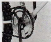
And here're those long buggers, the Ashtabula 7 1/2-inch cranks. Heat-treated, long, and strong.
