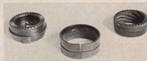
The retarder assembly, unassembled: (Left to right) drive-end expander, retarder spring, drive clutch.
