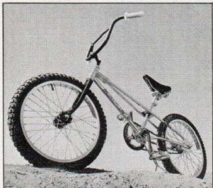
This is class machinery. Check the double top-tube frame construction. Low profile of the R&R RESULTS IN A LOW CENTER OF GRAVITY AND THE LOW C/G provides for amazing handling characteristics. Seat is definitely not moto.
