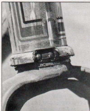
◀ The only thing to go south on the R&R was the lower bearing race on the steering head.
